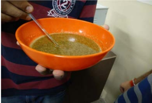
Figure 8. Mixing of Epoxy resin and Sugarcane Trash
