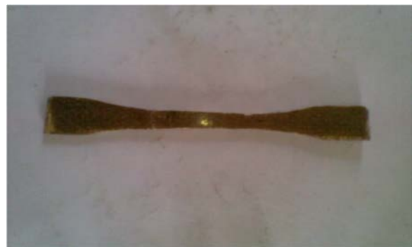
Figure 1. Tensile Test Specimen (Dog-Bone Type) line diagram
